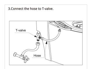
2. Existing water pipe connect T-valve.
