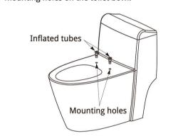
3. Place the Fixed Card on the toilet bowl where the mounting holes are. Make sure that the wash / dry gates are close to the rim and pointed down
