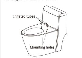
3. Place the Fixed Card on the toilet bowl where the mounting holes are. Make sure that the wash / dry gates are close to the rim and pointed down
