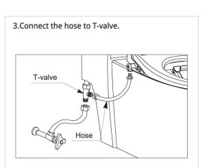
2. Existing water pipe connect T-valve.
